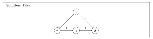
Consider the graph given above. The shortest path from c to d is (c,a,b,d) which is of weight 3. However, if the weight of each edge is increased by 1, the shortest path from c to d would be (c,d) of weight 5.
